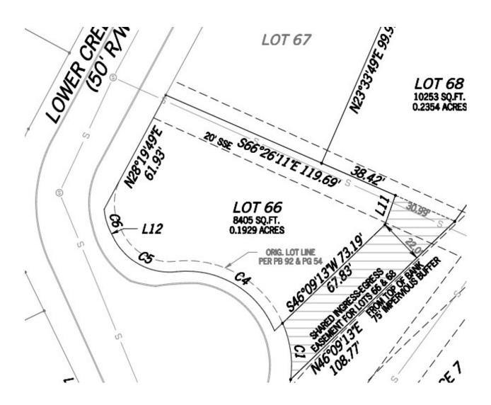
Shown above is the proposed re-platting for lot 66 to allow 5 feet less right of way along lot 66. The existing right of way is shown as a dashed line and the new line is shown as a solid line.
