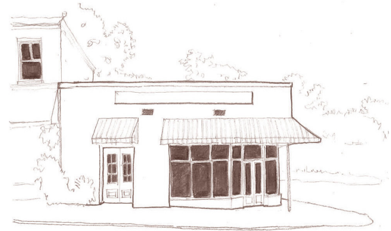
Awning Over Transom
