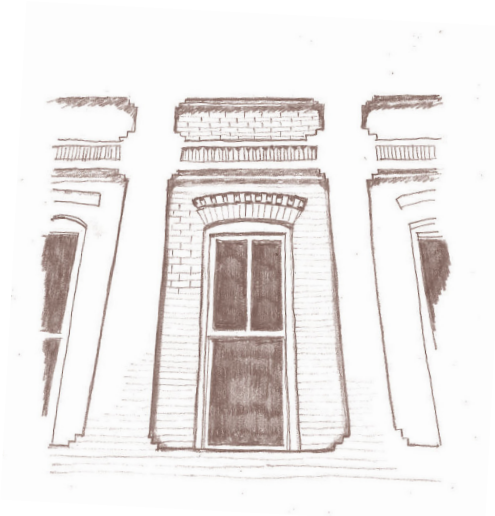
2:1 Window Proportion with Brick Arch
