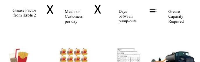
(1) To determine the correct grease factor, using Table 2, select the menu type (1 through 30), then the correct column (A through D) for whether there is a fryer and whether the establishment uses disposable or washable plates, glasses, knives, forks and spoons (flatware).
