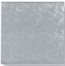
Acrylic Coated Galvalume TSR = 55%
