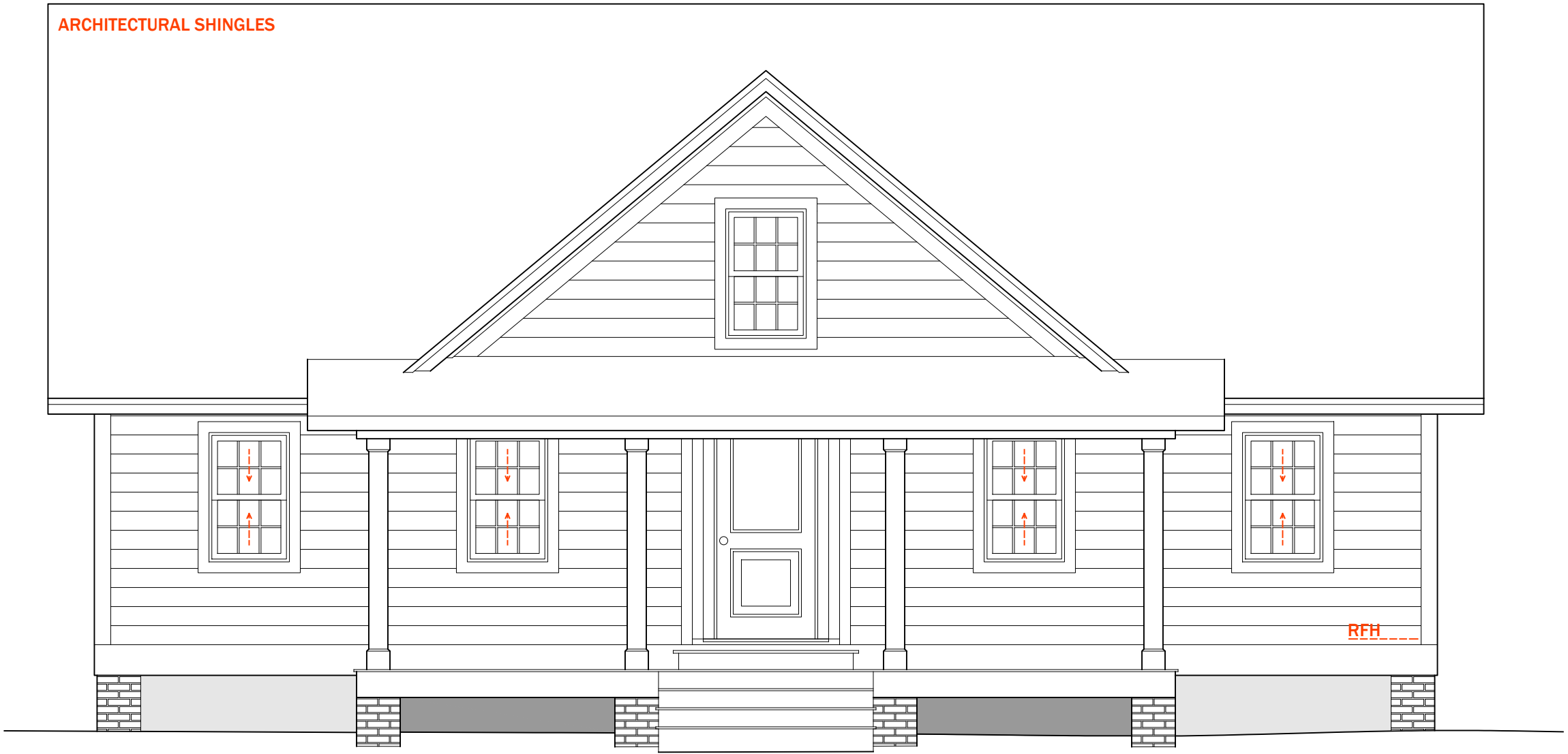
2.31 SOUTH ELEVATION SCALE: 1/4" = 1'
