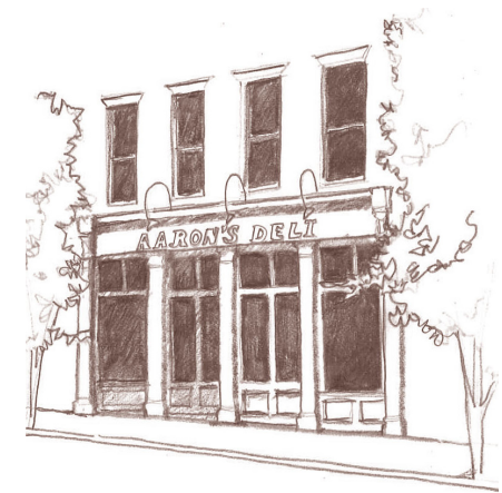
Sign on Flat Panel Above Facade
